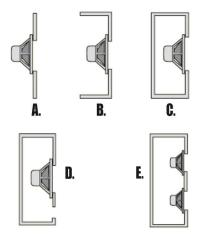
backwards" and then closed, to that an unwanted pressure compensation (=the "acoustic short circuit") is practically not possible any more. By doing this, it is possible to exploit the full (=maximum possible by the specific design) frequency spectrum for any specific loudspeaker system given.
