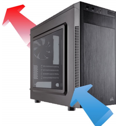
fig. 1. Exhaust fan: sucking warm air out of the chassis
